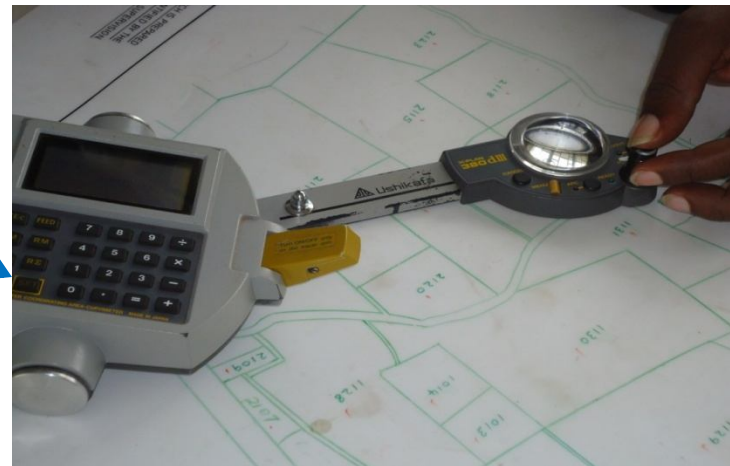
(7) Area measurement with plannimeter
