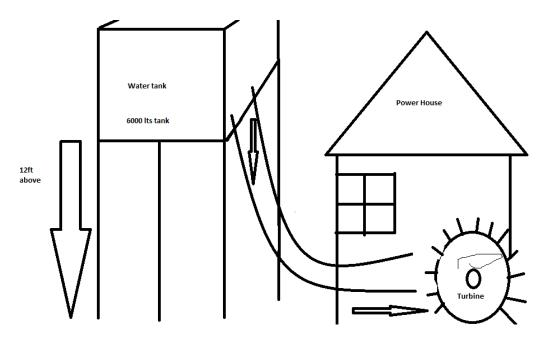
The generation involves tank raised 12ft above the ground with pipes running from the turbine. The turbine is then connected to the power house. A more detailed account is given below:
